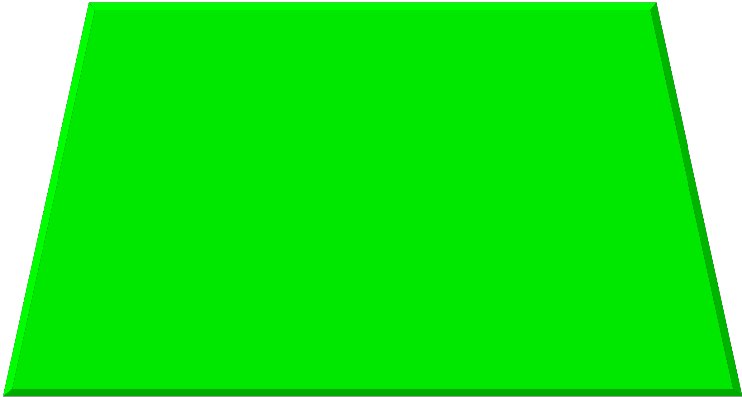
Shell large side make 2 .125 thick bevel edges 45 degrees
