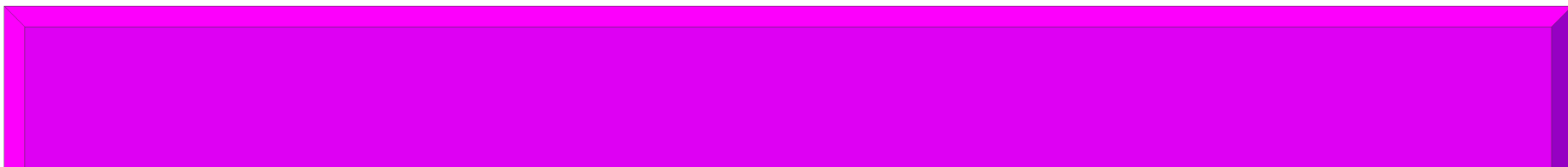
Shell top BBX side Make 2 .125 thick bevel edges 45 degrees
