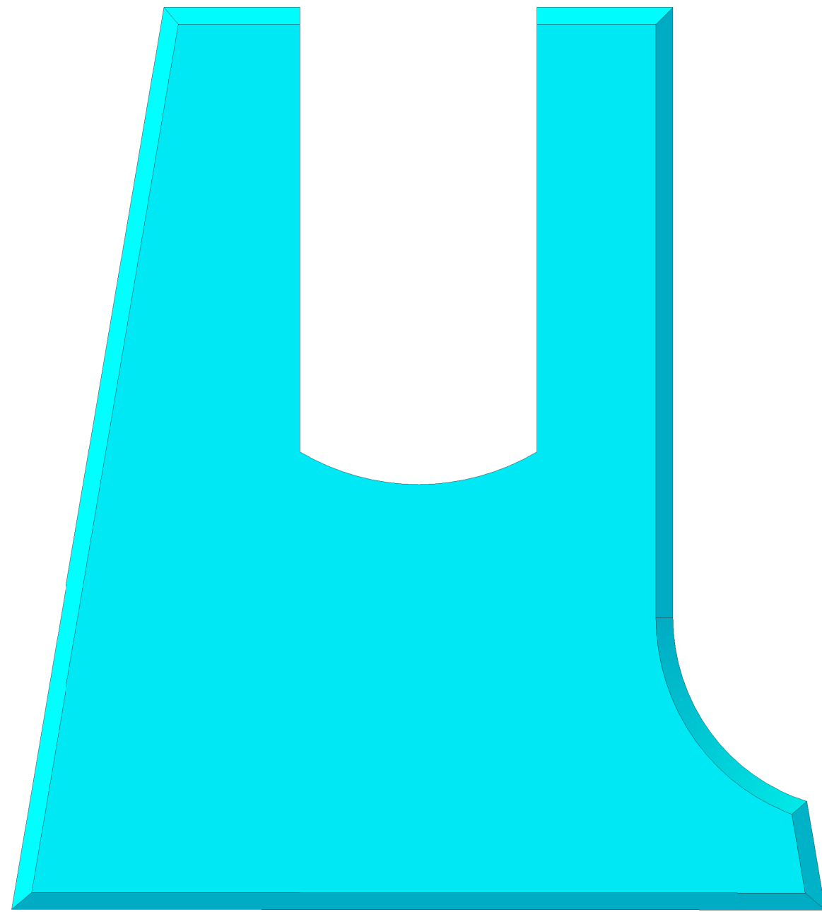
Shell left end make 2 .125 thick bevel edges 45 degrees
