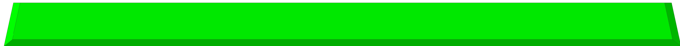
Shell BBX side bot make 2 .125 thick bevel edges 45 degrees
