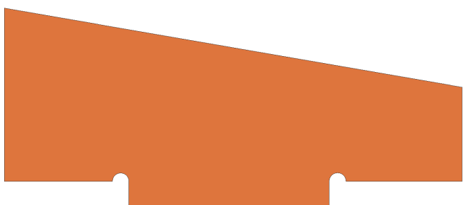
Shell Support make 4 .1875 thick
